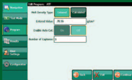
Fig. 6. Program creation screen for automatic time flow and time basis tests.
