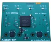
SyncBoard-9626 is available as a 2x or a 4x model: the 2x model allows a 2-board Master/ Slave system whereas the 4x model allows 2, 3 or 4 board Master/Slave systems.
