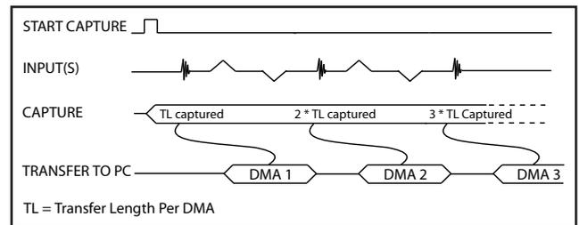
Continuous AutoDMA buffers do not include headers, so it is not possible to get trigger time-stamps.
