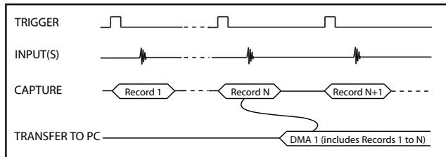
NPT AutoDMA is designed specifically for these applications. By only storing post-trigger data, the memory bandwidth is optimized and the entire on-board memory acts like a very deep FIFO.
