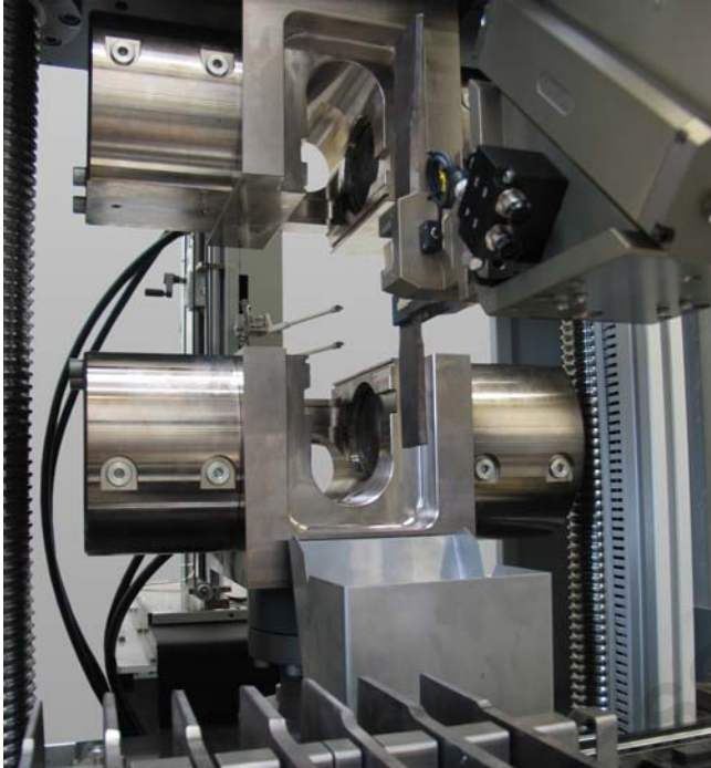
Feeding of the specimen to the testing machine
