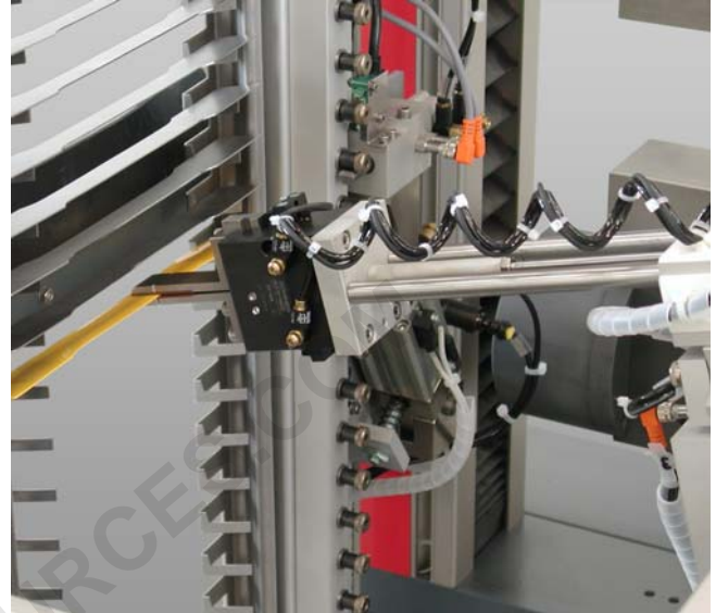
Pincer gripper removes a specimen from the magazine
