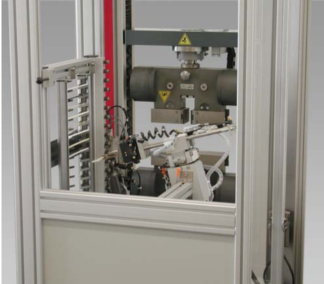
Working area of the robotic testing system 'roboTest A'
