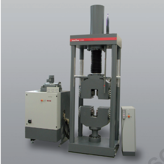
Figure: Zwick Z1200H with hydraulic grips
