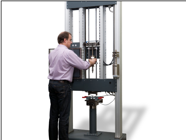
Amsler HIT 230F drop weight tester for pre-damaging plates (CAI)
