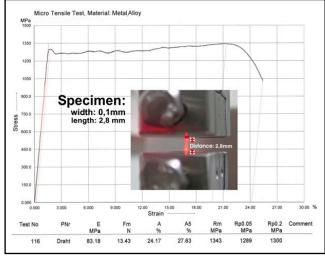
Strain-rate-controlled tests are also possible, as shown here on a micro-specimen.
