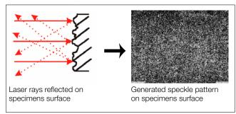
The specimen surface plus speckle patterns are recorded by a full-frame digital camera. Two evaluation windows are positioned within the overall image (= field of view) of the camera as virtual gage-marks. laserXtens tracks the speckle pattern in the virtual gage-mark using a sophisticated correlation algorithm between the individual camera image frames (speckle tracking).
