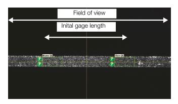
The algorithm operates in two different modes. As long as the virtual gage-mark moves within the field of vision of the camera, it will be tracked (=speckle tracking). As soon as the mark reaches the edge of the field of vision, changeover to a second measuring mode is available (= flow measurement). In this mode the flow of the
