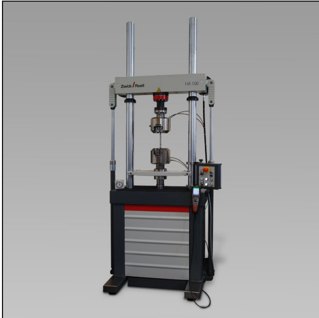
HA 100 on air springs with hydraulic wedge-grips
